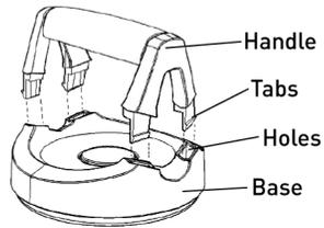
Place unit on a solid surface and push down in the middle of the Handle.
